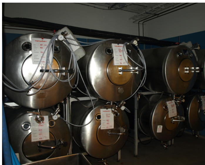
Figure 7.15 Fermentation of grape juice into wine produces \text{CO}_2 as a byproduct. Fermentation tanks have valves so that the pressure inside the tanks created by the carbon dioxide produced can be released.
